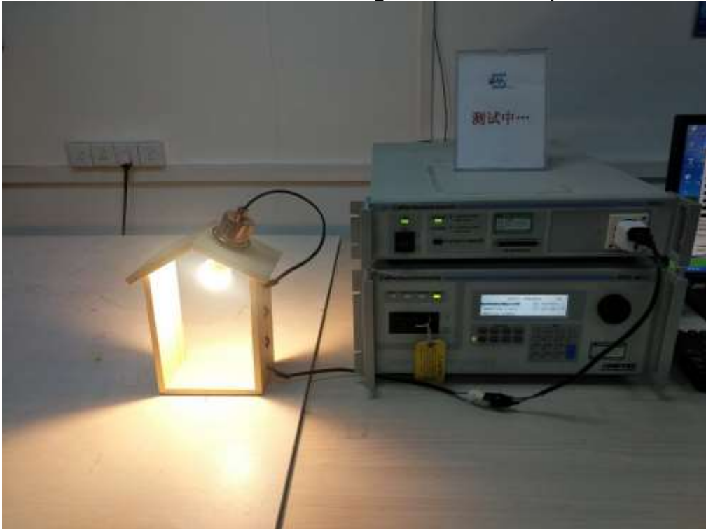
Current Harmonics /Voltage Flicker Test Setup
