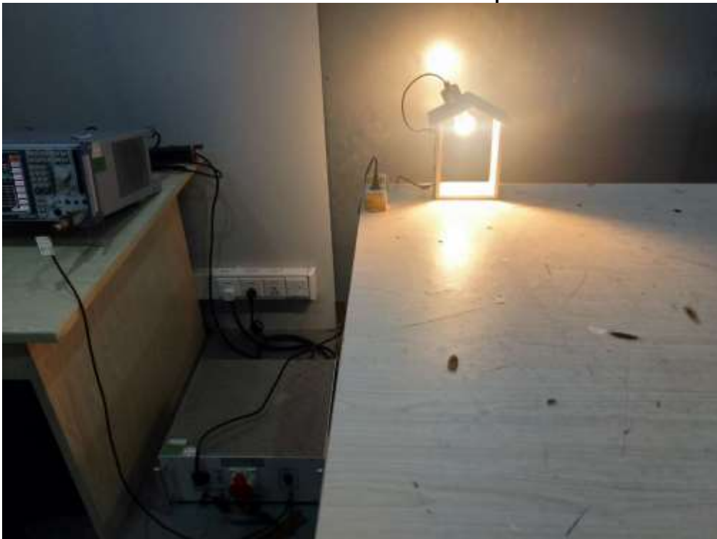
Conducted Emission Test Setup
