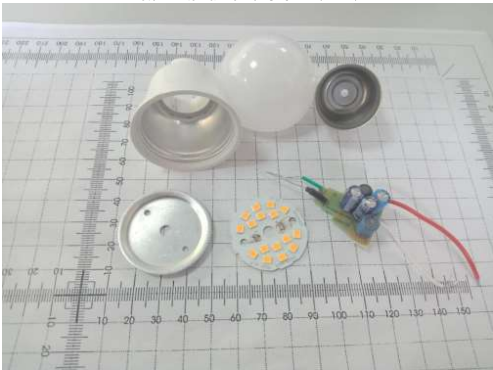
Photo 2: Internal view of G45-7-27/A12F/11
