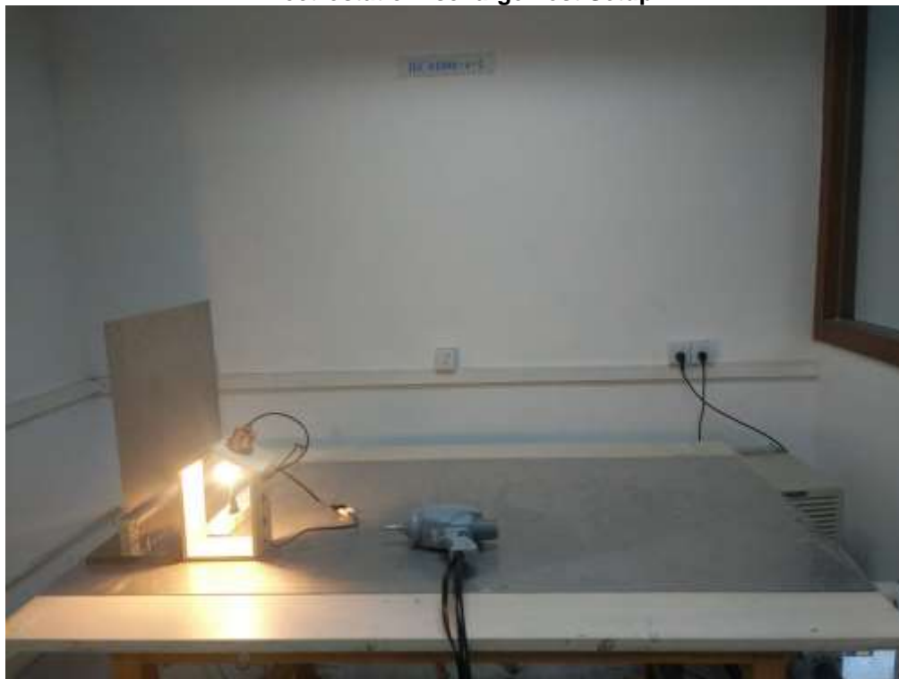
Electrostatic Discharge Test Setup
