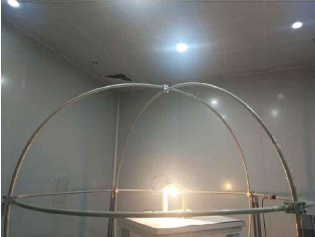
Radiated Electromagnetic Disturbances Test Setup
